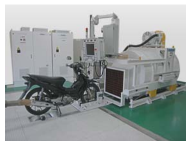
Emission test system
