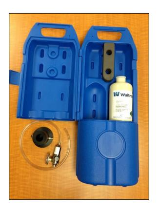
9065 Luminescent Dissolved Oxygen Analyzer Calibration Kit **Quick Reference Manual**
