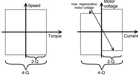
Regenerative (4-Q) power converter modules are used when motor torque can occur in either direction. This is for applications such as:
