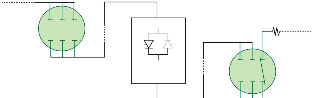
Either an AC or DC contactor is required, but not both.
