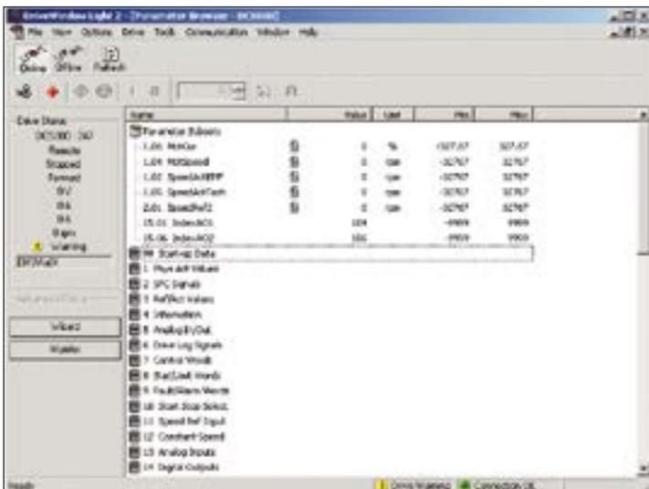
With DriveWindow Light, you can monitor up to four signals simultaneously. This can be done in both graphical and numerical format. Any signal can be set to start the monitoring from a pre-defined level.
