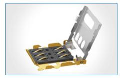
Mini UICC (Micro SIM) Connectors Amphenol's series of mini UICC connectors is designed to accept micro SIM cards for optimized printed wiring board area consumption. The mini UICC connector series features prevention of improper micro SIM card insertion or SIM card slide out. Different card handling possibilities include push-pull types, push lift / cover hinged types, bridge block or drawer versions.
