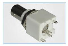
Valox Amphenol RF BNC Valox Connectors are isolated from the panel via a Valox housing to provide high performance in RF and microwave communications. BNC Valox Connectors feature a proven, easy-to-use interlocking interface that integrates seamlessly into any 50-ohm or 75-ohm RF system. These connectors are well-suited for instrumentation, broadcasting, and network applications.
