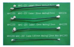
AMC Connectors, Jumpers and Adapters Amphenol Micro Coaxial (AMC) connectors, jumpers and adapters are ultra-low profile (2.5mm mating height) RF connectors with a small footprint (3mm x 3mm). The AMC series offers easy snap-on/off mating,  $50\Omega$  impedance, and DC - 6 GHz frequency range. The series is also 100% compatible with the U.FL interface.
