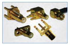
**SMC** The SMC connecter features a medium-sized 50  $\Omega$  threaded interface designed to meet of MIL-STD-348 standards as generated by the US Air Force. It utilizes die cast components on non-critical areas to provide a low cost solution. The series offers a 10-32 screw-on (threaded) coupling mechanism, allowing performance to 10GHz with low reflection.
