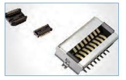
**BTB** Board-to-board connectors are available in plug-socket pairs with pin counts ranging from 8 to 50. Spring-type boardto-board connectors are robust and suitable for use in data center applications where there is the potential for external vibration.
