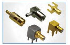
**SMB** Amphenol's SMB connectors conform to the requirements of Mil-C-39012, and the interface is in compliance with MIL-STD-348. Available in  $50\Omega$  and  $75\Omega$ , the SMB provides broadband capability through 10 GHz with a snap-on connector design and utilizes die cast components in non-critical areas to provide a low-cost solution.
