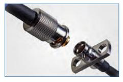
Quarterback The Quarterback® product line utilizes a high frequency miniature RF interface (up to 65 GHz) with a rugged bayonet coupling mechanism. The reduced withdrawal forces are well-suited for reliably mating cable assemblies to delicately soldered board mount connectors, minimizing potential PCB damage. Ideal for bench-top testing, high vibration environments, and high mating cycle applications.
