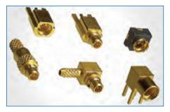
**MMCX** MMCX (also called MicroMate<sup>TM</sup>) is a micro-miniature connector series with a snap-lock mechanism allowing for 360-degree rotation. MMCX connectors conform to the European CECC 22000 specification. The MicroMate family of products is a 6 GHz 50  $\Omega$  interconnect. A range of connectors are available, including surface mount, edge card, and cable connectors. Common applications include broadband, instrumentation, and telecommunications.
