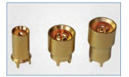
**AFI** The AFI connector interface is a solution for board-toboard RF applications. It utilizes a proprietary configuration that allows for industry leading "float" to compensate for the axial and radial misalignment due to packaging tolerances. This industry-leading float results in a maximum misalignment allowed by the system of .030" (0,8 mm) radial and .040" (1,0 mm) axial.
