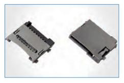
Memory Card Sockets Amphenol offers a full range of flash memory connectors (including SD, Mini-SD, Micro-SD, xD, CF1 & 2) with numerous features such as low-profile design, normal or reverse mounting, manual or push-push insert style, and a locking feature to prevent the card from dropping out. Available in SMT, straddle mount, or through-hole termination.
