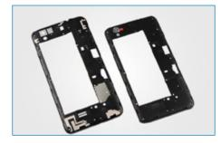
Mid Frame Antennas Amphenol designs and manufactures plastic mid-frames for smart devices utilizing custom insert molding for metal battery compartments, acoustic chambers, and other mechanical components. Two-shot LDS can be utilized for increasing mechanical strength of the frame yet create a unique LDS antenna geometry.
