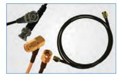
**RF Coaxial Cable Assemblies** Amphenol offers a full line of pre-assembled, fixed-length coaxial cable assemblies. Fixed length assemblies are for use in a variety of commercial and industrial applications that require standard configurations or lengths. Cables are available with popular connector series such as BNC, AMC, TNC, SMA and Type N.
