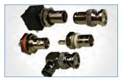
**BNC** Developed in the late 1940s as a miniature version of the Type C connector, BNC stands for Bayonet Neill Concelman and is named after Amphenol engineer Carl Concelman. The BNC product line is a miniature quick-connect RF connector. It features two bayonet lugs on the female connector. BNCs are ideally suited for termination on miniature and subminiature coaxial cable, including RG-58, 59, RG-179, and RG-316.
