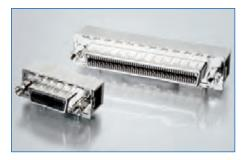
Infinity Connectors The Infinity series of receptacles is compliant with SFF-8470 specifications, and is available in both 4x and 12x configurations. Lanyard latching mating styles are available for use with CX4 and InfiniBand applications, as well as Screwlock mating styles for use with SAS, Fibre Channel and 10Gb Ethernet applications.
