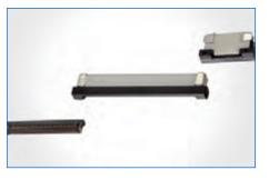
**FPC** Amphenol Flexprint connectors (C007 series) accommodate 0.3 mm thick flexprint cable with different contact configurations and pitch sizes. The double-sided, pre-stressed contact shape guarantees secure contact between the flexprint circuit and the connector, and allows insertion of the flexprint cable in either an upward or downward direction.
