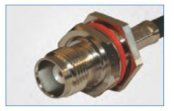
SC-Type Amphenol SC coaxial connectors are medium sized and offer constant  $50 \Omega$  impedance. They operate from 0-11 GHz and are manufactured to meet MIL-C-39012 specification. The connector mating is a .687-24 UNEF screw thread and the plug coupling nut has safety wire holes. Such qualifications make the SC interface ideal for military, instrumentations and testing applications.
