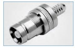
**1.6/5.6** Amphenol 1.6/5.6 coaxial connectors are miniature 75  $\Omega$  units operating from 0-1 GHz. The compact design of the 1.6/5.6 series permits dense connector packing, making these connectors ideally suited to applications where space limitation is a factor. Common applications include base stations, routers, and switching equipment.
