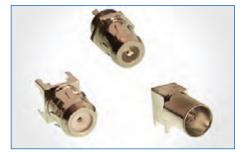
**Type G** Our Type G connector is a slide-on alternative to the Type F with 15A continuous current rating. The Type G complies with the MIL-STD 202 specification for vibration, shock, thermal shock, moisture resistance, and salt spray. The Type G has an impedance of 75  $\Omega$  — ideal for CATV applications. The Type G line consists of Bulkhead Mount Jack Receptacles and PCB Mount Jack Receptacles.
