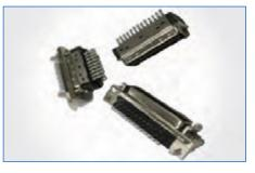
**MDR** Amphenol's MDR is a high-density shielded I/O connector with a broad range of board-mount, wire-mount, and cabling components. Ribbon contact is on a grid, which provides a small footprint connector, creating a reliable system for repetitive plugging and unplugging in I/O applications.
