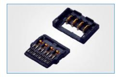
Battery Connectors Amphenol's comprehensive offering of battery connectors for mobile phones come in single and multicontact versions with straight and right angle mountings. They are available in a variety of pitches and heights to meet different phone and battery pad requirements. They feature stamp and form beryllium contacts with additional solder tags for high reliability and conductivity.
