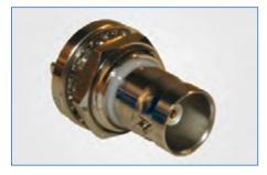
**Mini-BNC** The Mini-BNC is designed for wireless applications for higher connector densities while preserving the positive characteristics of the Amphenol full-size BNC's for 75  $\Omega$ systems., allowing 40% more interconnects in the same area. The Mini-BNC connector interface offers a 75  $\Omega$  impedance with acceptable return loss up through 1 GHz and a positive bayonet locking coupling mechanism.
