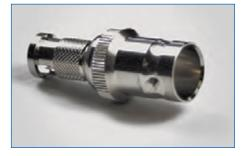
HD BNC HD BNC delivers true 75 ohm performance in a footprint 51% smaller than traditional BNC connectors, allowing four times the density. Engineered to enhance electrical and mechanical performance, the HD BNC connector features the trusted, push and turn interface of traditional BNC, providing tactile feedback and a positive lock for quick and guaranteed mating.
