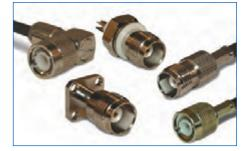
**TNC** The TNC connector series features a miniature, threaded weatherproof interface with a constant 50  $\Omega$  impedance and operates from 0 - 11 GHz. The TNC is available in standard and reverse polarity configurations. Reverse polarity is a keying system accomplished with a reverse interface, and ensures that reverse polarity interface connectors do not mate with standard interface connectors.
