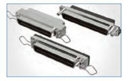
Filtered Connectors Amphenol's FCC57 series of filtered micro-ribbon connectors provides a very cost-effective solution to combat EMI. The family of connectors is the telephone industry's standard for multiple line connections. Available in 36, 50, and 64 sizes with a variety of termination styles, including: male/female, right angle PCB, vertical, press-fit, and solder cup.
