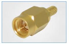
**SSMA** The SSMA connector is designed to be a space-saving alternative to the standard SMA originally designed for use with .085 semi-rigid cable. The male contact was designed to be the same size as the cable conductor so that it could be used as the mating pin for optimized VSWR. This interface is available with 50 0hm options and gold plating is standard.
