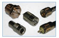
**UHF** Invented for use in the radio industry in the 1930's, UHF stands for Ultra High Frequency. While at the time 300 MHz was considered high frequency, these are now general purpose connectors for low frequency systems from 0.6 - 300 MHz. UHF connectors feature optional reducing adapters which accommodate a wide range of popular coaxial cables.
