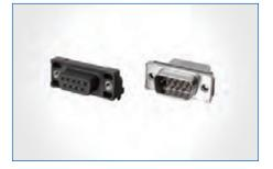
Harsh Environment D-Sub: MDB Series Amphenol's rugged D-Subs provide a cost-effective option for harsh environments. These environmentally sealed D-subs utilize high-performance thermoplastic inserts and metal die cast shells and are supplied with screw machine contacts. These connectors are available in both standard and high-density versions and a variety of termination styles.
