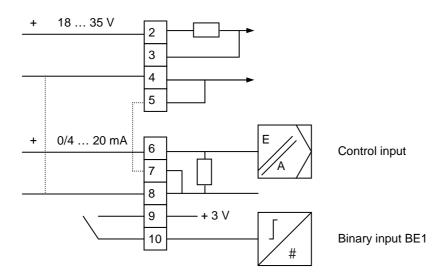
Figure 7 Electrical connection of 2/3/4 wire base device, 3/4 wire connection
