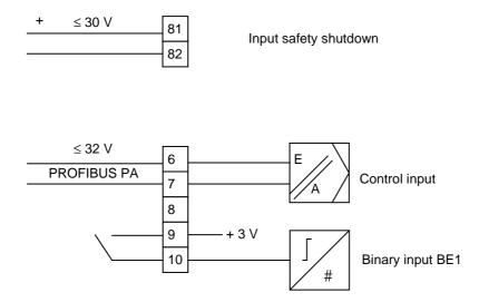
Figure 8 Electrical connection of base device, PROFIBUS PA
