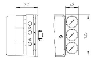
Figure 2 Dimensional drawing pressure gauge block
