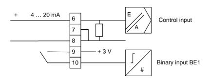
Figure 5 Electrical connection of 2 wire basic device
