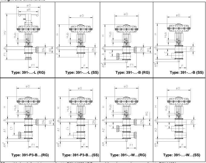
SS = welded ends for piping compliant to DIN 11850 / RG = round thread connections compliant to DIN 11851
