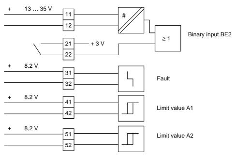
Figure 11 Electrical connection of binary module
