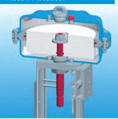
The universal diaphragm actuator, type UMA 811, is a product line comprising four sizes of actuator. The stem features a twin design and both interfaces for adapting to the valve are identical to facilitate toggling between the two directions. Instrumentation can be added by way of standardized NAMUR ribbing. An emergency override facility is available as an option.
