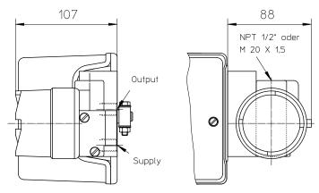
Figure 3 Dimensional drawing flame-proof type 824.D
