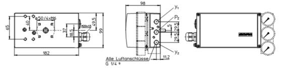
Figure 4 Metal enclosure, stainless steel
