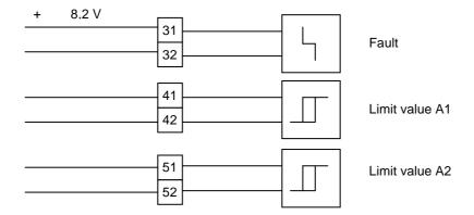
Figure 13 Electrical connection of contact module
