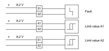
Figure 12 Electrical connection of slot initiator module
