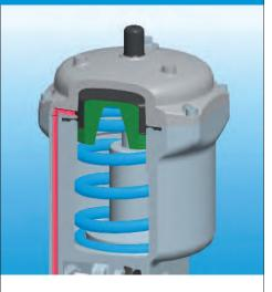
The ARCA-specific diaphragm enclosure and integrated air ducting have been integrated as a design feature. Characteristic for this pneumatic rotary actuator is the rolling diaphragm, which operates very uniformly with hysteresis-free torque output throughout the entire range. An emergency override can also be ordered or retrofitted.
