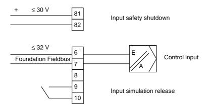
Figure 9 Electrical connection of base device, Fieldbus Foundation
