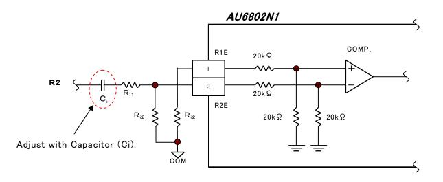
There might happen to exceed  $0V^{\sim}VCC$  range of R2E terminal voltage, and it cause some failure. Then the terminal voltage for R2E should not exceed  $0V^{\sim}VCC$  by means of adding the external resistor ( $R_{i1}$ ,  $R_{i2}$ ) to divide the voltage.
