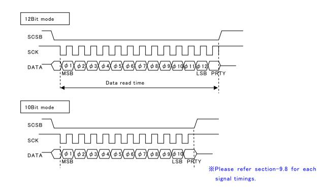
OPRTY is defined as even parity. The number of "1" data between " $\phi 1 \sim \phi 12$ " and "PRTY" must be even.
