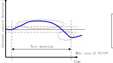
There is an abnormal R/D conversion situation (control deviation exceed the threshold), and if such situation is over 50% of test duration, it is detected as fault.
