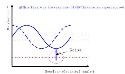
Due to a noise, monitor output cross the threshold down. Then it is detected as fault.
