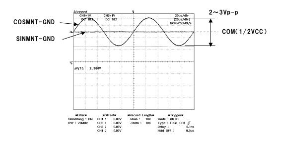
%If potential difference between SINMNT and CONMNT generate by the deviation of R<sub>1</sub>, it cause a error source. Please select appropriate resistor grade according to your system tolerance.
