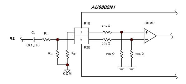
In this dual power source case, an exciting signal is 0V center. So it needs to make R1E/R2E terminal input level as shifting DC level. There might happen to exceed 0V<sup>°</sup>VCC range of R2E terminal voltage, and it cause some failure. Then the terminal voltage for R2E should not exceed 0V<sup>°</sup>VCC by means of adding the external resistor( $R_{i1}$ ,  $R_{i2}$ ) to divide the voltage.
