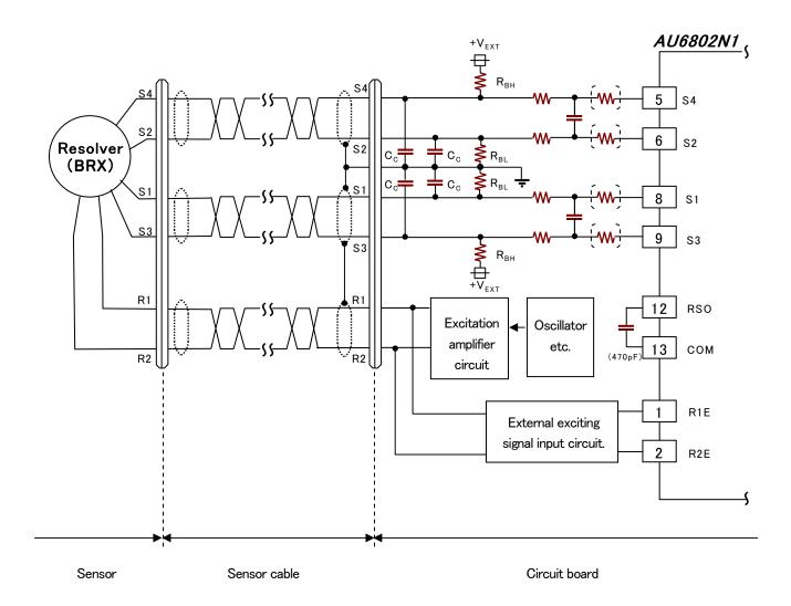
Connection example: Used external oscillator as excitation source.
