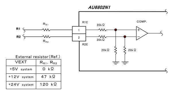
In case of direct input for R1E/R2E, exciting signal level might exceed VCC and it cause some failure. So please note that the terminal voltage for R1E/R2E should not exceed VCC(Power supply voltage) by means of adding the external resistor ( $R_{R1}$ ,  $R_{R2}$ ) to divide the voltage.
