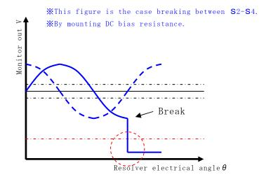
In case of breaking signal line, monitor output will be less than threshold DC level and it is detected as fault.
