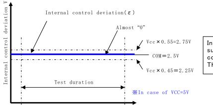
In the state that have been successfully R/D converted, control deviation is almost "0". Then it is not detected as fault.
