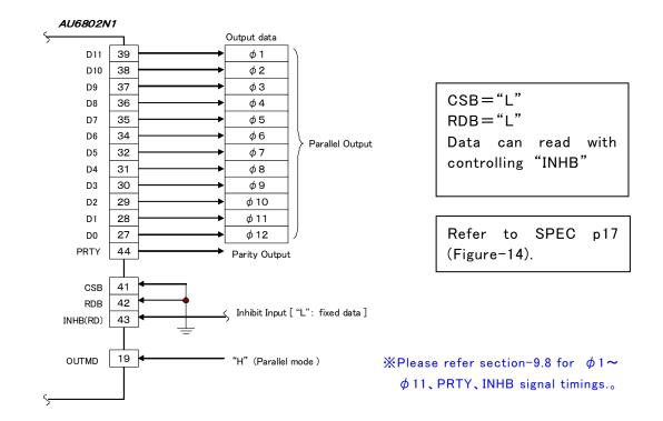
■Parallel BUS interface mode《Bus output》: interfaced by BUS line
