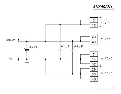
Power source is single supply  $+5V \pm 5\%$ . Analog power line and Digital power line can connect to same power line. If you set separate power line for analog(VCC) and digital(VDD), there must be no potential difference between VCC and VDD, or AGND and DGND. Also power switching (power-on or power-off) should be done simultaneously.
