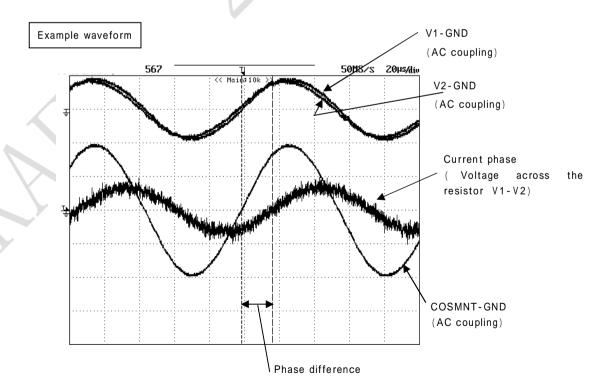
The above example is for the phase advance case of voltage monitor signal.
