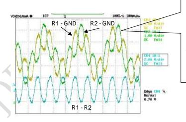
It might happen to have R1-GND/R2-GND oscilation due to OP-AMP characteristic. If this kind of wave is observed, DC cut Capacitor (Ci) might cause unstability of DC current. Then insersion of resistor between Ci output and GND will be effective to stabilize it.
