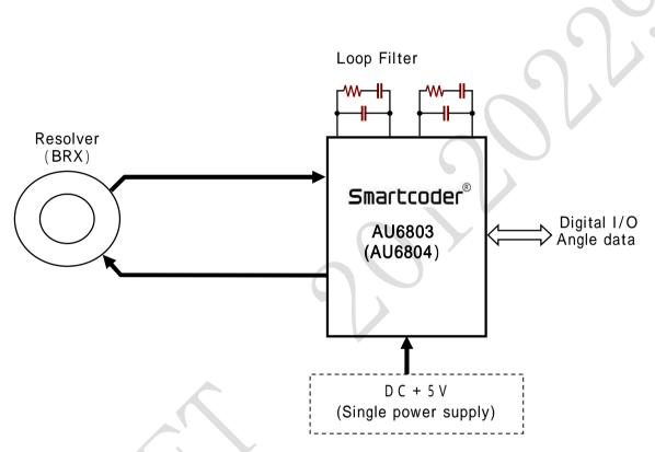
Some applications will require an external clock input and separate excitation amplifier.
