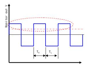
When the monitor output is in a rectangular wave to be saturated, it will be " $T_H$ = $T_L$ " condition then it might be detected as fault situation due to boundary conditions for the determination.
