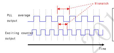
When PLL unlocked and R/D conversion is not performed normal, the phase relationship between PLL average output and exciting counter output has changed and frequency is getting mismatched. Then it is detected as fault situation.
