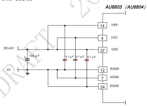
Power source is single supply  $+5V \pm 5\%$ . Analog power lines(VCC/AGND), digital power lines (VDD/DGND) and excitation power lines(VRR/RGND) must connect to each of the same one. If you set separate power line for VCC-VDD - VRR or AGND-DGND - RGND, there must be no potential difference and power switching(On/Off) should be done simultaneously.
