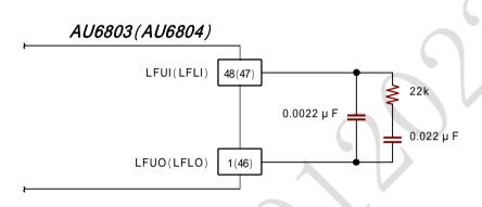
Regarding loop filter connection, please connect wiring compact as much as possible with given the constant of resistor and capacitor. Especially input terminals (LFLI, LFUI) must be carefull not to enter noise due to sensitive terminals.
