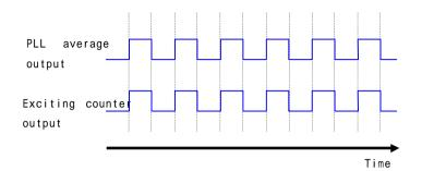
In normal R/D conversion state, PLL average output value and exciting counter output (frequency) are matched. Also phase maintain a certain relationship. Then it is not detect as fault.
