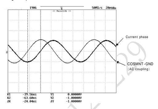
Phase shift[°] = 360[°] x (Time shift[μs] / Exciting frequency period[μs])
