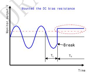
In case of breaking signal line, the monitor output DC level will exceed threshold value due to DC bias resistance and this " $T_H > T_L$ " situation can detect as fault.
