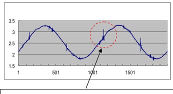
Basic waveform (10kHz) was not changed much. But spike noise was overlapped.
