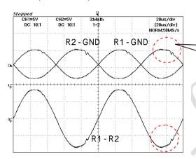
The wrong constant selection cause wider amplitude, and waveform distortion will be occurred by OP-AMP or Tr saturation voltage, etc. Need to avoid distortion.
