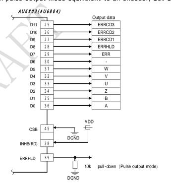
A,B,Z pulse which come from D0 D2 pins are same signal with dedicated A,B,Z pin (42 44 pin).
