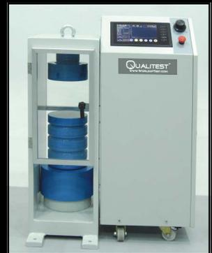
Exceeding of the ASTM C-39 standard provisions (starts with the 10% of the machine capacity), QCRT-AC series of Automatic Compression Testing Machines are supplied in Class 1 starting from 50 kN. This exceptional performance enables the machines to be used for a considerable number of applications including:
