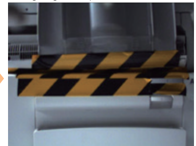
Fig.2 After measures (with shielding tapes) A-weighting sound pressure level: 62.6 dB
