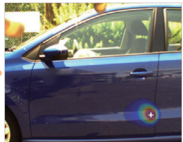
B Door hitting sound (rear lower of the front door) (Analyzed in 8 to 12 kHz)*
