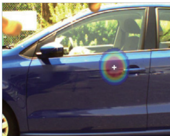
A Door latching sound (rear upper of the front door) (Analyzed in 8 to 12 kHz)*
