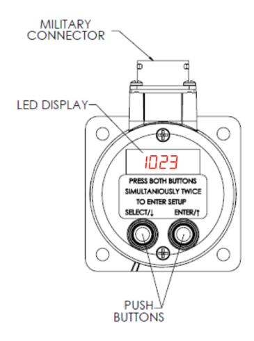
The EZ25 Encoders have two modes of operation: **Run Mode** and **Programming Mode**.
