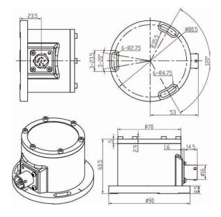
Picture1 Housing with MIL class connector
