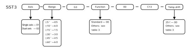
For example, if order a dual axis CAN inclinometer, with range  $\pm 15^{\circ}$ , room temperature accuracy  $\pm 0.02^{\circ}$ ,  $-20 \sim 60^{\circ}$ C accuracy  $\pm 0.02^{\circ}$ , output CAN2.0, 25 meters cable with plug, GPS function module, the model should be chosen as: SST302-15-G3-F1 -00-C13-D3 (25m)
