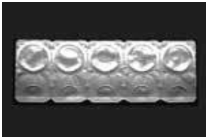
With visible light lighting, it is difficult to detect the contact lenses.
