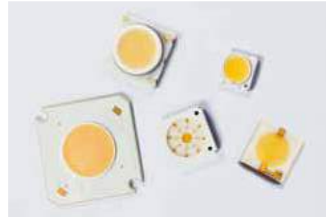
① Correlated color temperature: 2,800 K, General color rendering index: Ra 97
