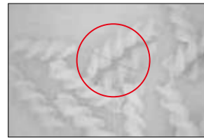
It is possible to form an image of the foreign material using infrared light.
