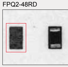
Film glare is removed, making it possible to determine if the part is there.
