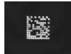
It is possible to determine the 2-D code by evenly illuminating the surface.
