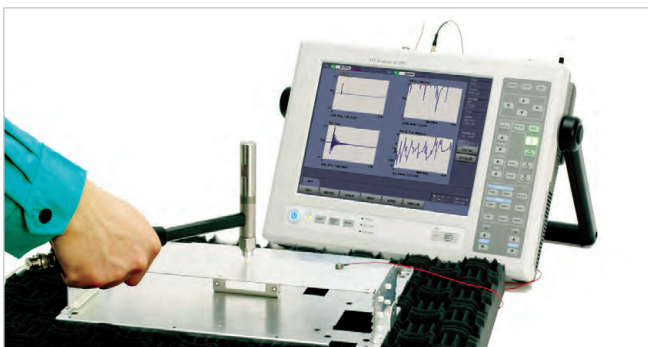
Hammering measurement with the CF-7200A, the GK-3100 Impulse-force Hammer and the NP Series Accelerometer
