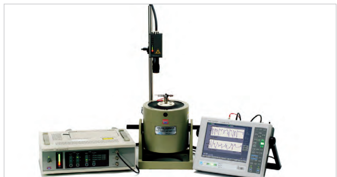
Analysis of micro-object using the LV Series Laser Doppler Vibrometer and a magnetolectric shaker
