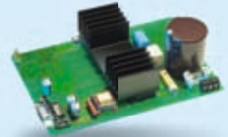
Motor control for washing machine
