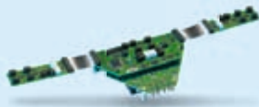
Customer-specific cooktop control with combinatorial circuit part
