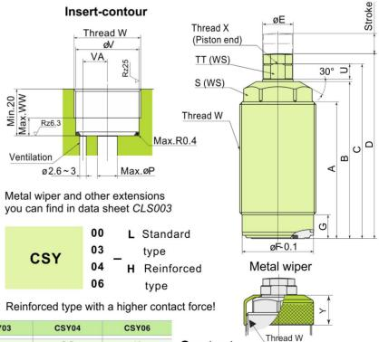
CSY03 CSY00 Support force 3 5.5 Oil demand (cm3) 0.6 0.8 1.2 2.0 L : Standard (N) 2 ~ 4 4 ~ 6 5 ~ 8 5 ~ 8 Spring contact force H: Strong spring (N) 3 ~ 6 5 ~ 8 6 ~ 11 8 ~ 14 Stroke (mm) 6.5 8 8 10 0.05 maximum weight thrust piece (kg) 0.2 0.3 0.4 0.7 (kg)
