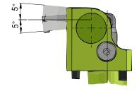
In order to create the maximum clamping force and minimum transverse force, a variation of the horizontal clamping position of the lever of a maximum of +/- 5  $^\circ$  is recommended.
