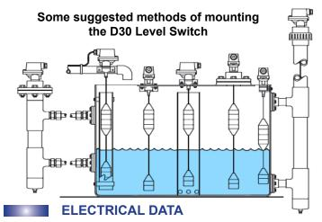
The D30 level switch contains a high capacity single pole double through microswitch with tungsten contacts, specifically designed to control motor loads up to 2 Horse Power
