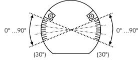
\* Working range of 90° can be reduced up to 30° from each end position.
