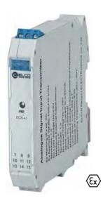
Transmit single/double channel thermocouple signals or voltage signals in the hazardous area by isolating and transmitting output single/double current or voltage to non-hazardous area. It has cold junction temperature compensation function and can be connected to a connection network in non-hazardous area via communication interface. It is an intelligent product with online self-diagnosis function. Customer may set the input signal type and output range with a handheld programmer.
