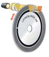
are common, which is very exacting in terms of optics. They must be manufactured with optimum precision and no contaminants – therefore production takes place in a cleanroom.
