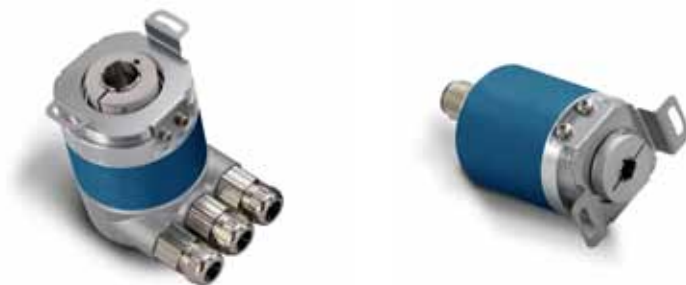
Avtron absolute models: (left) HS6A w/15mm bore and 3X cable entry "K" option; (right) model HS6M w/6mm bore, tether, and axial M12 connector option "A"
