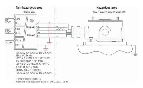
Picture 2 Barrier & wiring diagram
