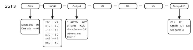
For example: If ordering need an explosion proof inclinometer, measurement range is  $\pm 5^{\circ}$ , the accuracy is  $\pm 0.02^{\circ}$  (normal temp) ,  $\pm 0.02^{\circ}$  at temp from  $-20 \sim 60^{\circ}$ C,  $4 \sim 20$ mA output, 10m length cable, so the model should be SST302-05-G19-00-B5-C9-D3 (10m) Options (see table 4):
