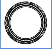
**Optical Disc for Incremental Encoder**
