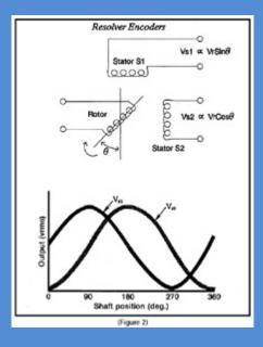
A Ratiometric Tracking Converter features a Type II servo-loop that comprises of a sine/cosine multiplier and an error amplifier together with phase sensitive demodulator, error processor, voltage controlled oscillator (VCO) and an up/down counter. The information produced by this type of converter is always "fresh", being continually updated and always available at the output. The basis of determining the shaft angle in a ratiometric converter is the ratio between the two stator signals:
