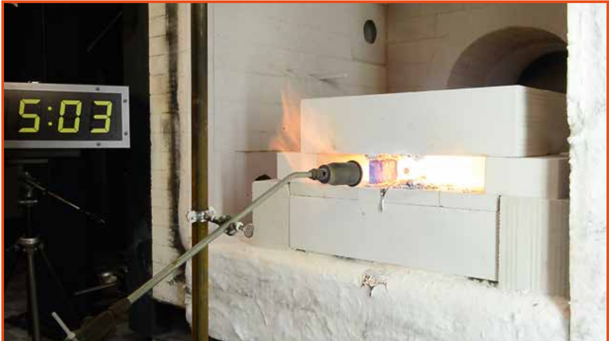
At 5:03 minutes the melted aluminum dripped of the bottom of the re-circulation chamber.
