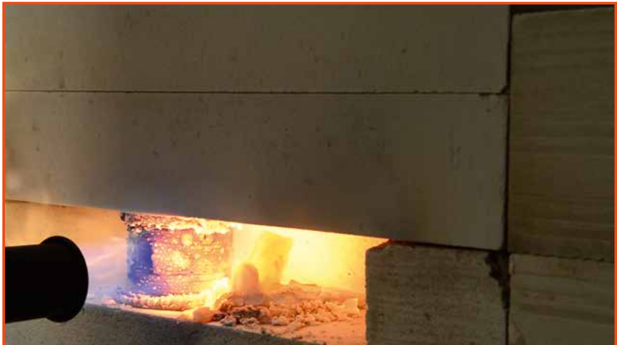
Close-up of the FISSIC® coating after almost 10 minutes testing. The coating holds together and does not fall off.
