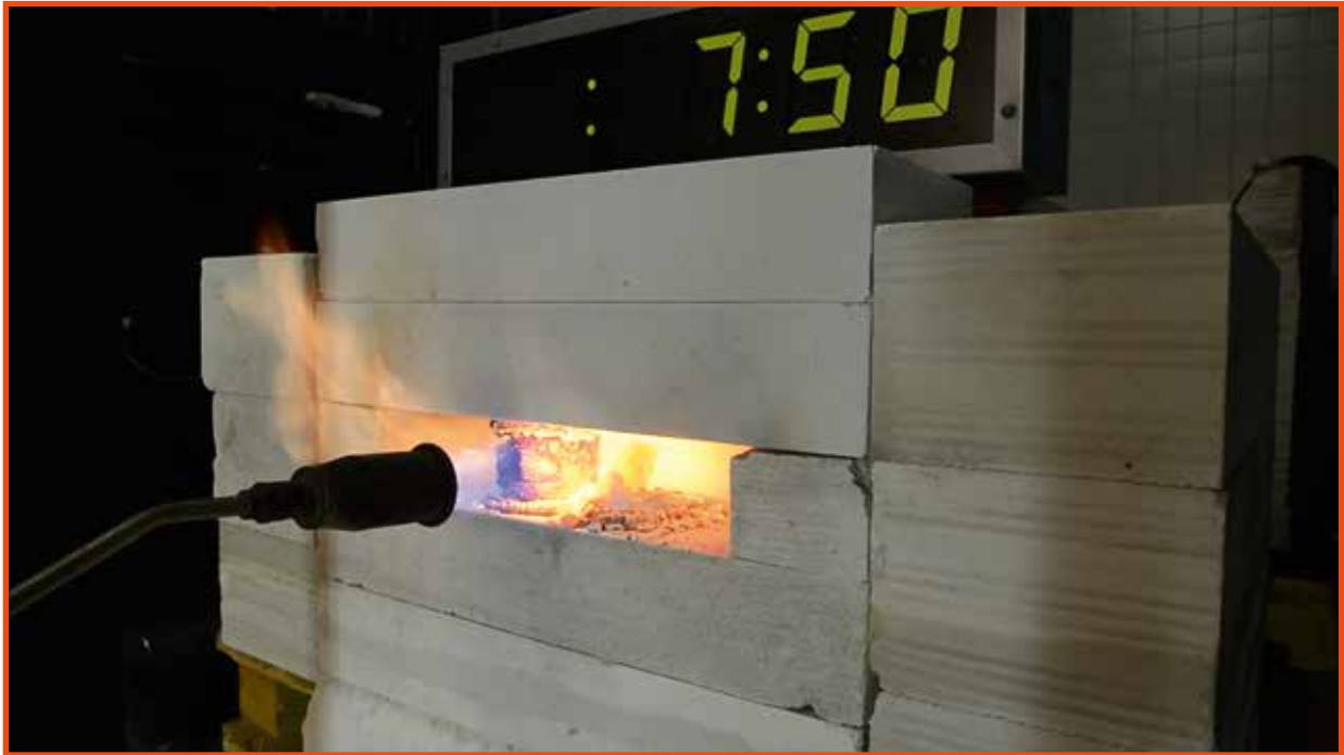
After the aluminum has burned away, leaving reminders on the floor, the intensified flaming disappeared.
