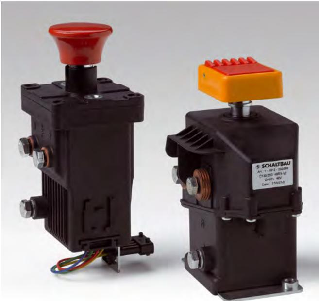
Schaltbau's competitively-priced all-in-one device is a combination of line contactor, main fuse and manual cut-off switch in which additional devices as well as an optional horn can be integrated. Typical applications are battery powered warehouse machines, such as fork lift and reach trucks as well as walk-behind trucks and stackers.
