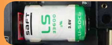
Internal lithium battery
