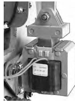
Example of 81,000 Series pin, spring and spacer requirements for vertical above mounting.
