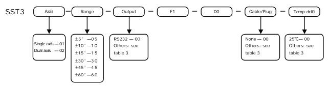
For example, if order a dual-axis GPS inclinometer, with range  $\pm 30^{\circ}$ , accuracy  $\pm 0.02^{\circ}$ at room temperature and  $-20-60^{\circ}$ C, CAN2.0 output, 2m cable, the model should be chosen as: SST302-30-G3-F1-00-C1-D3 (2m)
