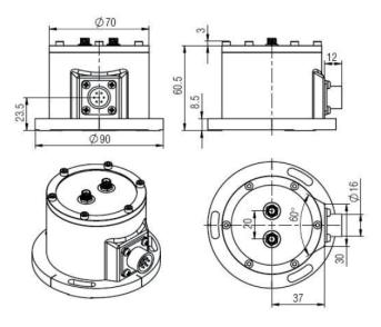
Picture 2 Housing with MIL class connector
