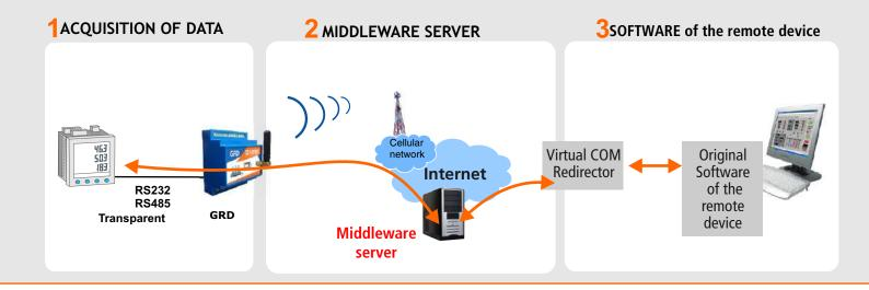
**SCADA Seral port mode:** Consults are made in Modbus, DNP3, or IEC101 protocols, between the devices connected through the serial ports of the GRDs. This mode uses the Demultiplexing feature.
