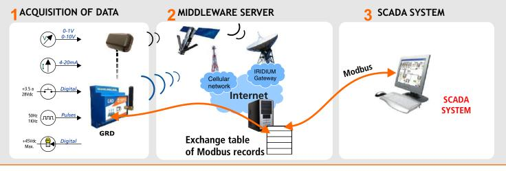
**SCADA Serial port:** This form consults, in Modbus, DNP3, or IEC101 protocol, the devices connected through the serial port of the GRDs. In this way the devices' demultiplexing feature can be used.
