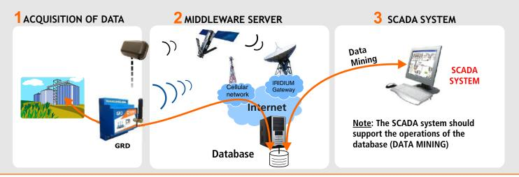
**SCADA I/O:** The SCADA System consults directly, in Modbus protocol, for the records of the GRD devices; consulting about the state of the inputs and outputs.
