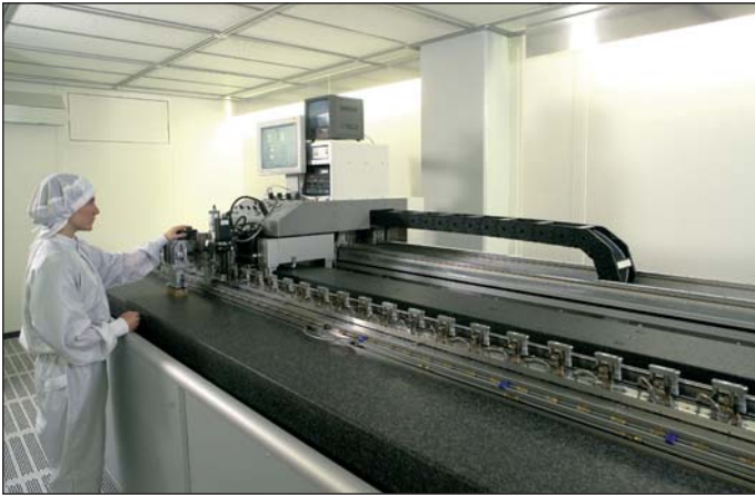
Measuring machine for linear scales
