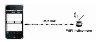
Picture 1 Access to one Wi-Fi Inclinometer
