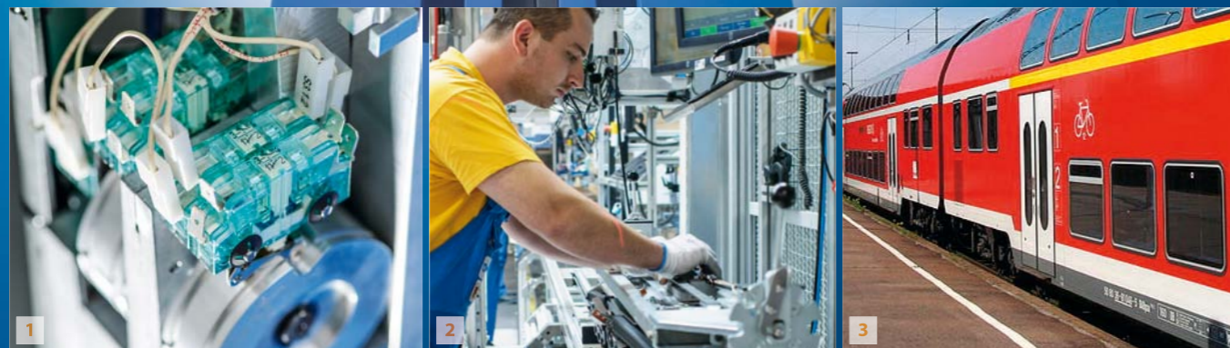
1 Emergency unlocking device on the door drive unit | 2 Serial production was taken up in the manufacturing plant even before the market launch | 3 An IFE E4 access system installed on a double-decker coach of Deutsche Bahn
