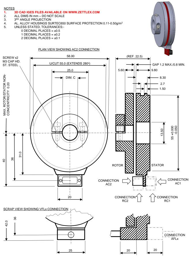
OPTIONS FOR DIM C = 6.00, 10.00, 12.00 & 12.70 ALL WITH H7 TOLERANCE. OPTIONS FOR CONNECTOR = AC1, AC2, RC1, RC2, AFL1 T0 5, VFL1 TO 5 - SEE SECTION 8 ON HOW TO SELECT BY PART NUMBER.
