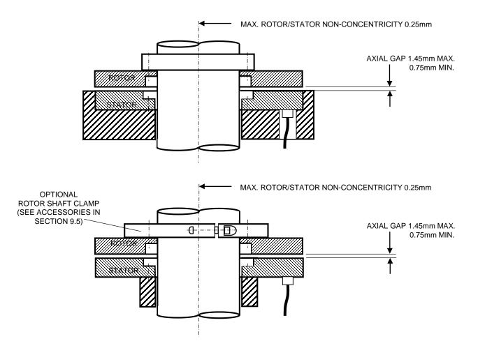
All formats of IncOder can be installed using a circumferential clamp in the host equipment. This applies to Rotor or Stator. Preferably the C-ring's gap is closed by at least one screw.
