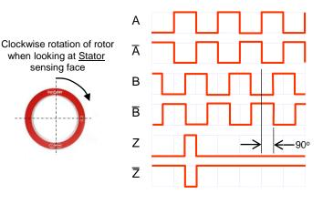
A leads B for clockwise rotation of rotor Phasing: 90° electrical Symmetry: 180° electrical Max. pulse frequency: 1MHz High signal: >2.5V Low signal: <0.5V Max. output load: 30mA Diagram shows 90° width Z reference (ABZ1)
