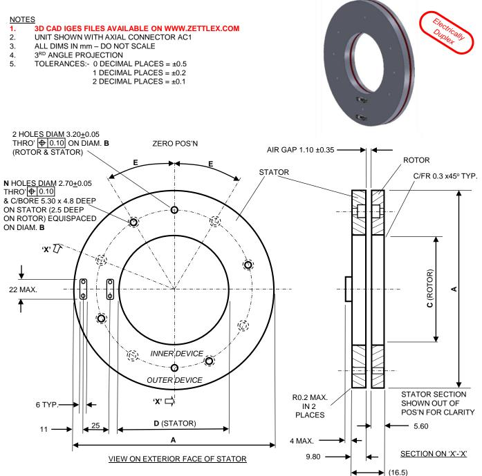
Duplex IncOders are electrically redundant:- 2 electrically independent IncOders in 1 package – the first on the outer annulus, the second on the inner. The range starts at an O.D. of 125mm with axial connections (AC1) or integral flying leads (AFL1-5). Note - measurement performance is quoted for the outer annulus device.
