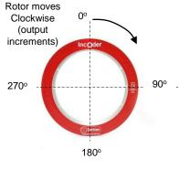
View on Stator Sensing Face
