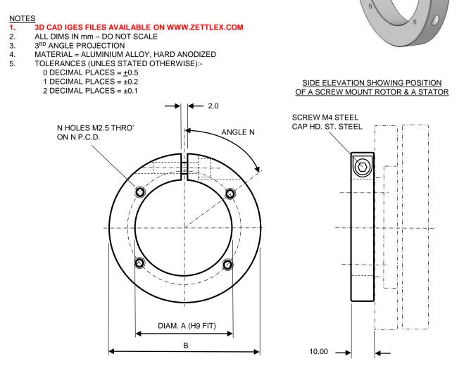
NOTE REGARDING ATTACHMENT METHOD. FIRSTLY, ATTACH CLAMP TO ROTOR USING 'N' SCREWS. TIGHTEN M4 SHAFT CLAMP SCREW TO SECURE TO SHAFT AND ONLY THEN TIGHTEN THE 2 SCREWS ADJACENT TO SHAFT CLAMP SPLIT LINE.
