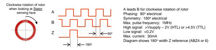
Note: 1 edge = 1 count or 1 bit. 4 counts per pulse. Readers should be set to 4x resolution for full resolution.
