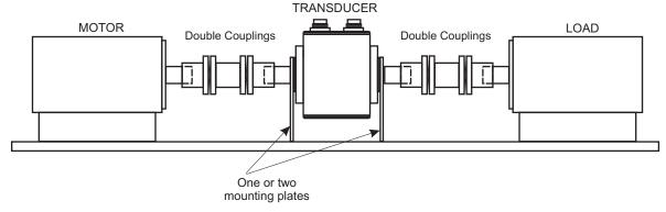
For rotary torque transducers **with torque ranges 1Nm (10lbf.in.) or less**, it is recommended that the transducer is rigidly mounted using the tapped locating holes on the end caps of the transducer. Care should be taken not to induce any end loads or bending moments to the shaft, as these may induce inaccuracies to the torque measurement and in extreme cases damage the transducer.
