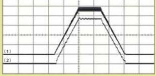
The output shows driving pulse(1) and the hunting of the motor(2).
