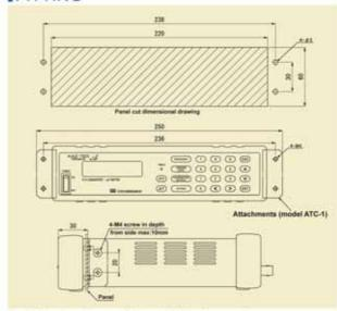
A pair of Attachment for panel fitting (model ATC-1) is as a option.
