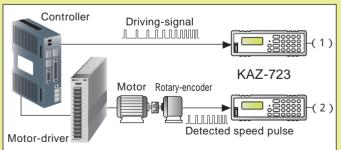
CONDITIONS KAZ-723(1) Mode: F/V mode Settled Full scale Frequency: 70kHz Settled Analogue output: 0 to 10V
