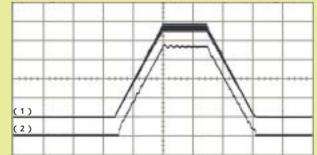
The output shows the jitter contained driving pulse and the hunting of the motor.
