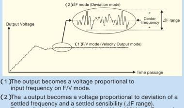
The applicable center frequency is  $1\text{Hz} \sim 100\text{kHz}$ .  $\angle F$  range has 6 steps 0.5%  $\sim 20\%$ .
