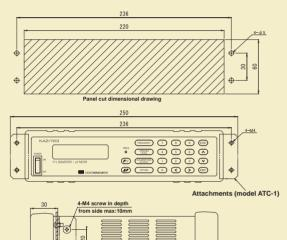
A pair of Attachment for panel fitting (model ATC-1) is as a option.
