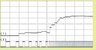
CONDITIONS KAZ-723(1) Mode: E/V mode Settled Full scale Frequency: 150Hz Settled Analogue output : 0 to 10V Input Signal(2) Input Frequency: 0 to 100Hz Oscilloscope Time axis : 100ms/div Voltage axis (1): 2V/div. Voltage axis (2): 10V/div.
