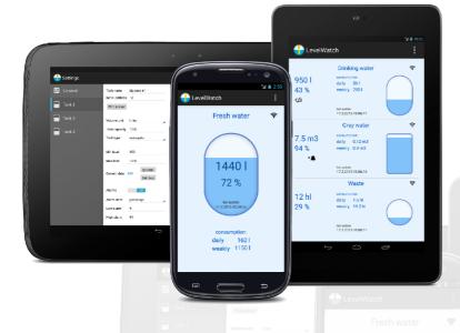
Levelwatch BLE-C is capacitive wireless tank level monitor for smartphones. Sensor continuously measures the level and sends data to smartphone via Bluetooth. Data from sensor is monitored by using free application on smartphone or tablet. Very useful are information about daily and weekly consumption. Sensor is suitable for water and other water based liquids.
