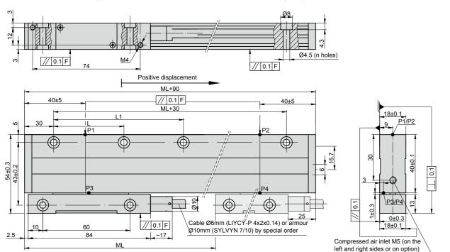
F - Machine guideway ML - Measuring length P - Gauging points for alignment
