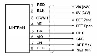
'Set Max' and 'Set Min' are factory settings and should not be connected without prior consultation with Zettlex LINTRAN factory settings are with 0% and 100% at the extremes of the measurement range.
