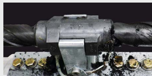
Conventional well-proven IFE screw drive
