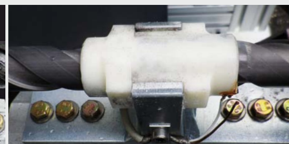
New lubrication-free IFE screw drive
