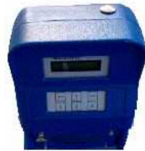
View of the MC108: keyboard, display and outlet RS485 for remote terminal TRM100 in the top part.
