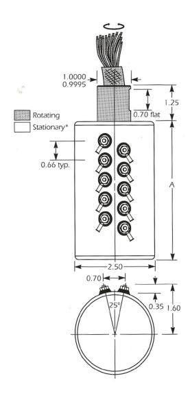
\*Housing can rotate (shaft held stationary) if RPM's are low or if unit is balanced by Meridian Laboratory.
