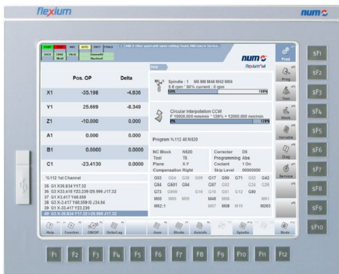
Panel with 22 Function Keys Reference with PC Panel coding "F"
