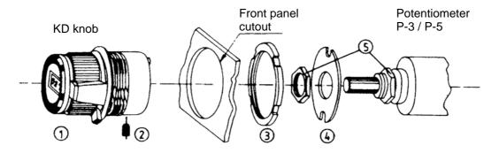
Proceed as follows to assemble/install the potentiometer:
