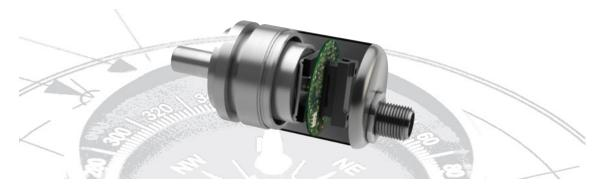
Magnetic rotary encoders determine angular position using magnetic field sensor technology. A permanent magnet fixed to the encoder's shaft creates a magnetic field which is sampled by a sensor that generates an accurate absolute position reading.
