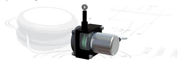
POSITAL's LINARIX draw wire sensors measure linear motion by displacing a retractable stainless steel wire wound around a cable drum that actuates the rotary encoder coupled to it. The encoder then provides a proportional output. Measurements are highly accurate, reliable and the systems have very long lifetimes.
