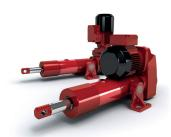
Rolaram linear actuators comes into their own when high precision or performance actuation is required or as a replacement for a hydraulic or pneumatic units. There are 8 standard models, available in 2 standard drive configurations. Roller screw design are available for the highest performance applications and ball screw designs when less performance is required. Custom designs are available.
