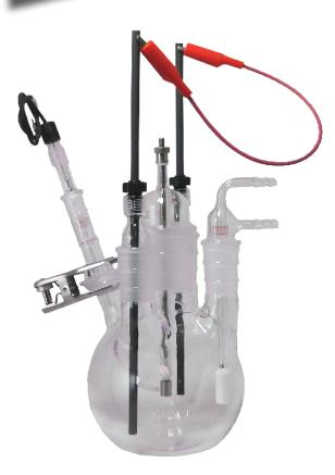
The K0047 is ideal for testing and evaluation of metal specimens in corrosive environments. It is fashioned after a well-known cell configuration and is a standard in some ASTM methods.
