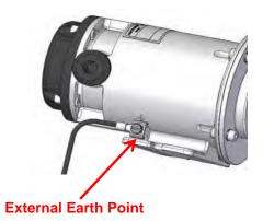
The detector housing must be connected to local ground via the external earth point. The wire should be minimum 4 mm2 (8 AWG) and as short as possible.
