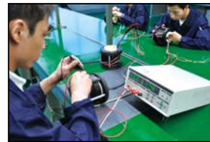
绝缘测试 Insulation Test
