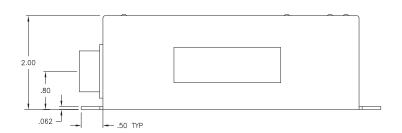
J1:5PIN\_ A +INPUT (18VDC-40VDC) B COMMON RETURN C + OUTPUT (0VDC-5VDC, 0A-8.2A) D CONTROL (0KOhm-5Kohm) E SP ARE
